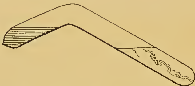
FIG. 7.—Faraday's Tube for Liquefying Carbon Dioxide.
